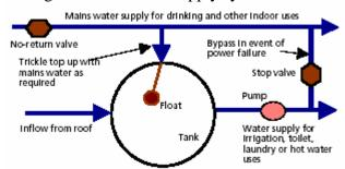
Note that the non-return valve is to be a testable backflow prevention valve.
