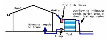
Configuration of a gravity system:
