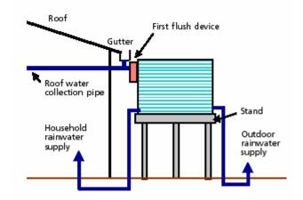
Storage components of a dual supply system:
