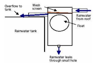
Suggested plumbing configuration for rainwater tanks in urban areas with a reticulated supply – direct connection with potable supply.
