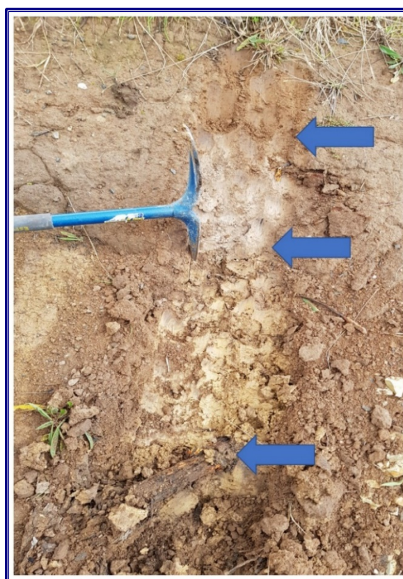
Figure 8 – Soils and Geology Typical texture contrast soil on the slopes of the Showground, showing hard-setting reddish brown sandy clay loam topsoil (0 – 100mm), massive sandy clay loam pallid zone (100 – 250mm), mottled yellowish clay subsoil merging into weathering. sandstones of the Flagstone Formation (700mm+).
