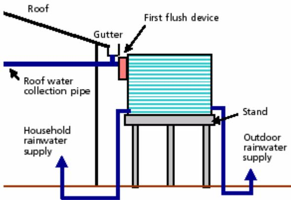
Storage components of a dual supply system:
