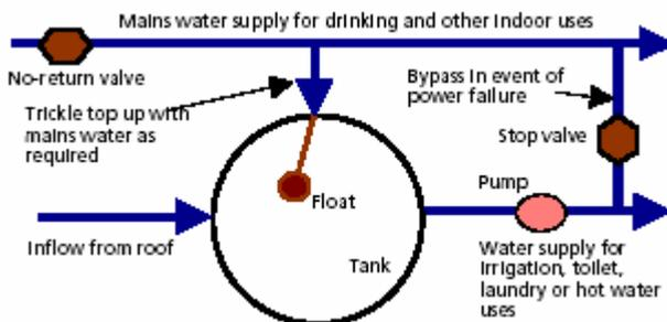
Note that the non-return valve is to be a testable backflow prevention valve.
