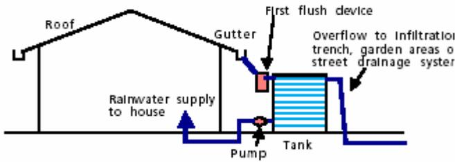
Configuration of a gravity system:
