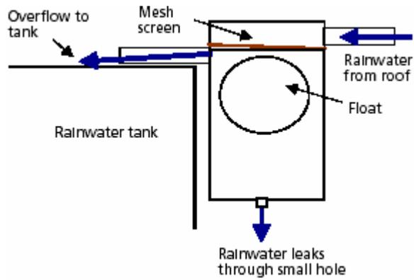
Suggested plumbing configuration for rainwater tanks in urban areas with a reticulated supply – direct connection with potable supply.
