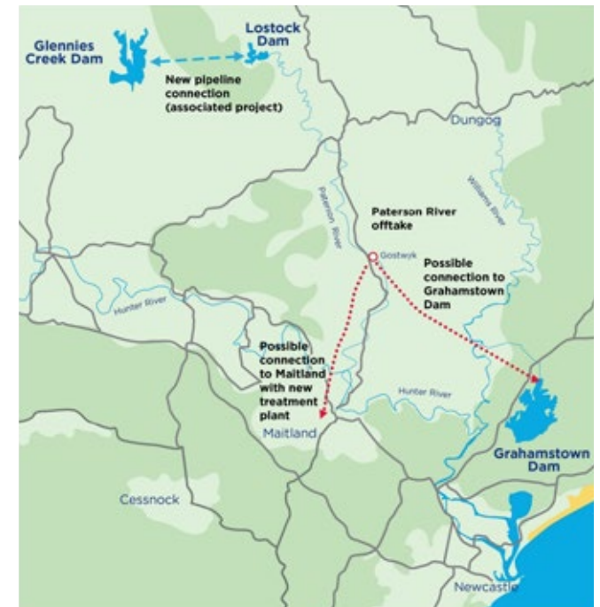
Figure 2 – Map of the proposed Lostock Dam – Glennies Creek Dam pipeline scheme and Hunter Water Connection (Hunter Water, 2022. Lower Hunter Water Security Plan)
